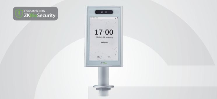
**Elite Pass** is a fast and accurate facial recognition terminal adopting deep learning algorithm that can be installed on and is compatible with entrance products such as flap barriers, swing barriers, tripod turnstiles of ZKTeco and the third parties.
